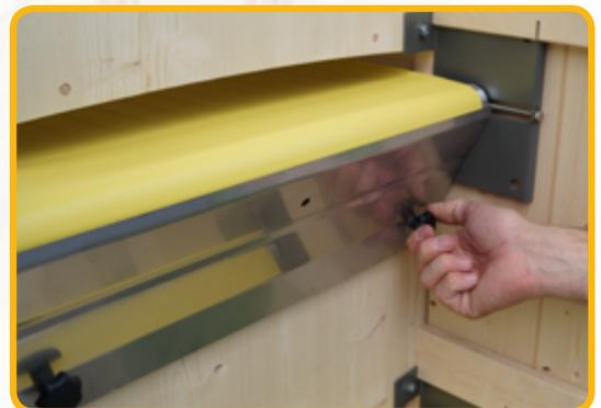
Fit the scraper blade and firmly screw it on.
