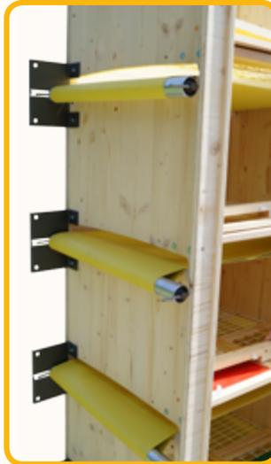
Feed the return shaft complete with the screwed-in screws through the droppings belt up to and into the rear bearing plate. Important: The connecting joints of the shafts must always point outwards.
