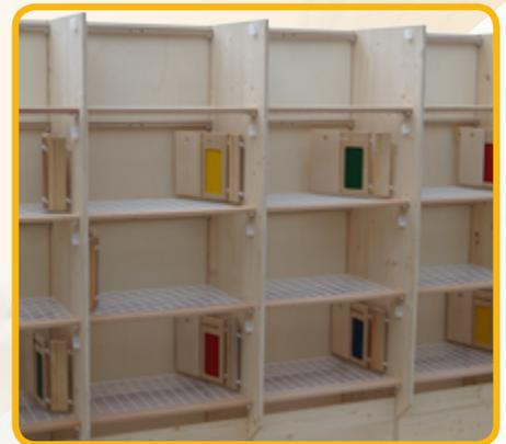
Fit the front doors with the hinge onto the hooks of the upright side panels.
