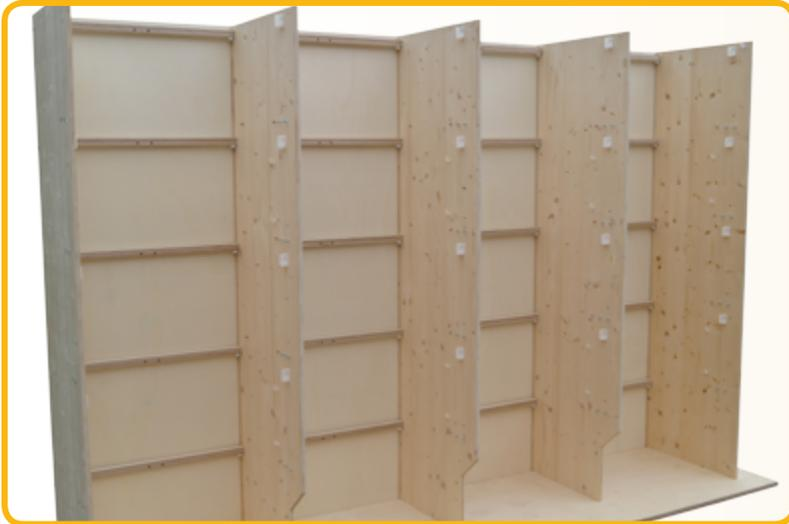
If the box is delivered with a rear panel, insert the panel in the grooves at the back of the sides. Then, from the top to the bottom, push the rear crossbars with the dimensions 19 x 27 mm onto the metal bolts on the side panels. 5 bars in total. In doing so, the holes in the rear crossbars must always be facing forward.
