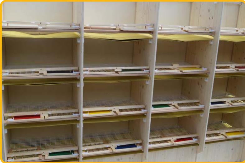
Arrange the front bars with the four plastic hooks in the sections. Important: With the section sizes 69.2 cm, 59.2 cm and 54.2 cm, the bars are marked with the numbers 1 and 2. The bars with the number 1 are fitted in the top section rows. The bars with the number 2 are fitted in the second row from the top and so on.
